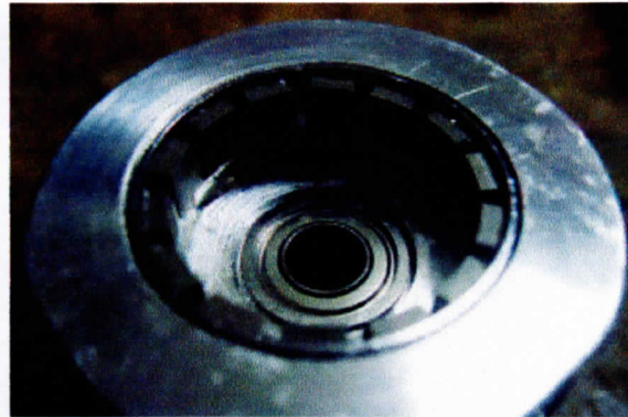
Figure 15. Pressed-in bearing and glued rotor.
